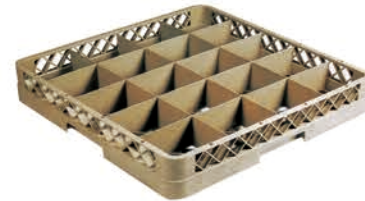
16K29709 20-Compartment Glass Rack Art.No: T-20 Overall Size: L500xW500xH100mm Comp.size: L115xW95xH80mm Material/Colour: PP/Beige Packing: 6pcs
