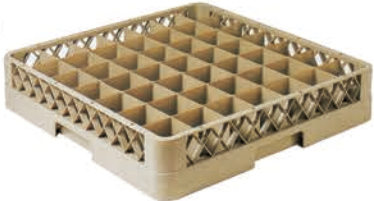
16K29711 25-Compartment Glass Rack Art.No: T-25 Overall Size: L500xW500xH100mm Comp.size: L90xW90xH45mm Material/Colour: PP/Beige Packing: 6pcs
